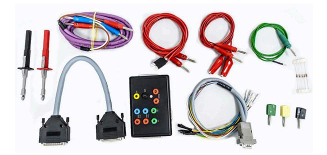
The ZN051 Distribution Box is used mainly with the Abrites Diagnostics software for Mercedes. However, one of it's features is the capability to connect your AVDI through BOOT MODE in EDC17 ECUs found in VAG vehicles.
