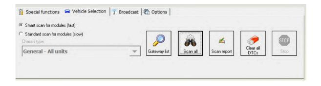
Standard scan – the software is iterating through all possible units and is trying to establish connection to them. This was the only one scanning mode prior software version V24.
