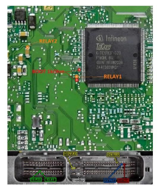
On Different EDC 17 ECUs, you can follow the following steps to connect to the ECU when using the ZN051 Distribution Box.
