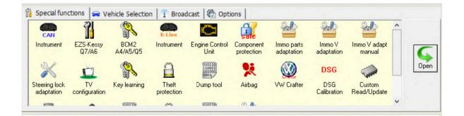
The needed special function is opened by double click or by marking and clicking the "Open" button.
