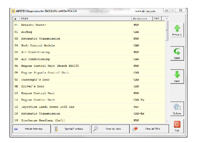
This is the main screen of the software and it shows all the navigation buttons as well as the ones for vehicle selection, scanning and general diagnostic trouble code (DTC) clearing.
