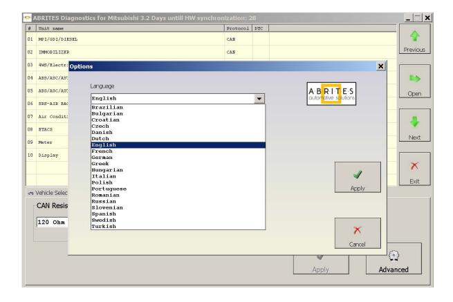
When a control unit is connected, you can make identification, Read DTCs, Clear DTCs, display Actual Values, make Actuator Tests, edit the module coding and get access to many "Other Functions" the different vehicle models and modules you are connected to offer. Here's an example of how the menus look like:
