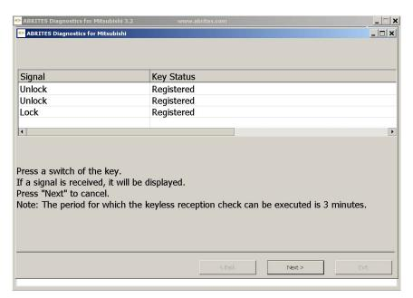
The PIN code of the vehicle will be automatically generated once the procedure is started. Before proceeding with the key programming function, you should make sure that you are using the correct transponder chip. The transponder in the key should be HITAG (PCF7936). It should be configured to work in Password Mode. The transponder can be configured by using the "Tag Key Tool" software.
