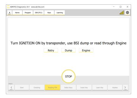
If you decide to load a dump of the BSI, you can read it by soldering to specific points of the unit, and reading it on bench. You will need an <u>ZN030 Abprog programmer</u>, and a <u>ZN057 Wire Extender</u> for Abprog
