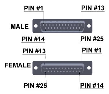
Here is how to use the DB25 adapter as some of the additional adapters intended to work with ABProg programmer:
