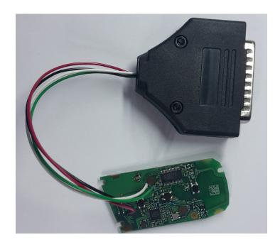
You can connect the adapter to the ABPROG adapter to AVDI as shown in the picture below:
