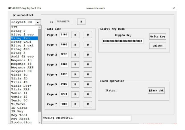
You have also the ability to access additional EEPROM memory of the keys, to prepare a key ready for starting of the vehicle using 'Key Tool', to prepare transponders ready for programming by diagnostic equipment – 'Production' and also you can prepare a 'cloning' of a key using function 'Key Cloner'.
